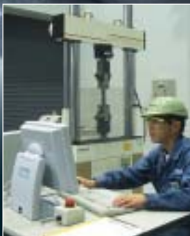
Chain fatigue test
