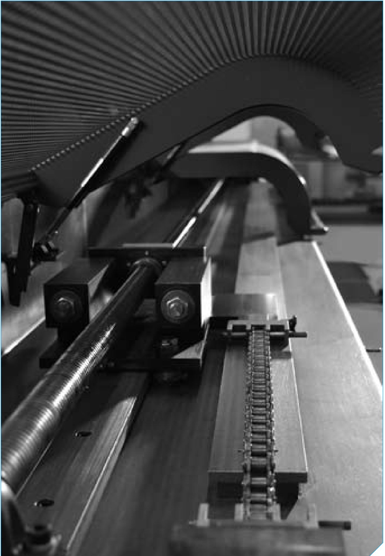
Chain Length Measuring Equipment (the "Matchy")
