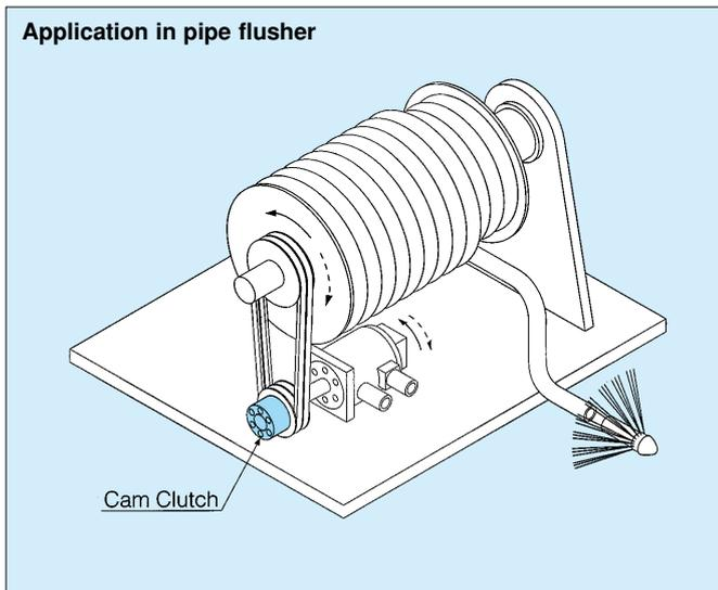
**A-2-3. Application for the purpose of selectively driving either one of two driven units by normal or reverse rotation of the drive input (see the figure below)**
