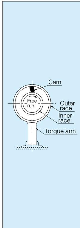
Prevention of reverse rotation of inclined and vertical conveyors is a typical example of how backstopping is used. The following A, B, and C types are available for different Cam Clutch mounting positions, and the series listed are designed to handle each specification.
