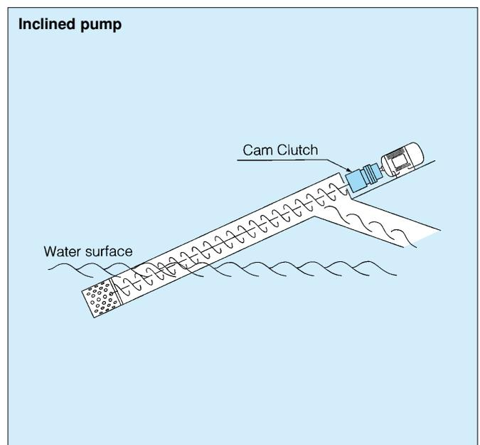
**A-2-2. Application for the purpose of braking the driven side (see the figure below)**
