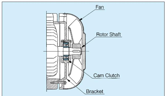
This example shows a Cam Clutch installed to a motor pulley to prevent reverse rotation. Cam Clutches can be installed to inclined belt conveyor systems to prevent reversing when the conveyor stops, as a result of power loss or other causes.
