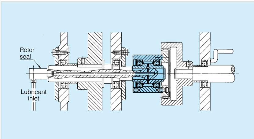
In some situations the Cam Clutch might be installed deep within your equipment making routine maintenance very difficult, or even impossible. The diagram on the left shows one such example.
