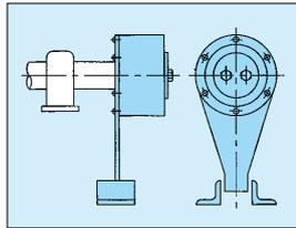
Since reverse rotation is prevented directly by the conveyor shaft without using a drive chain, gears, or couplings, this is regarded as the safest and most reliable mounting method. Additionally, a low overrunning speed minimizes the cam overrunning slip speed, as well as the overall slipping distance. As a result, wear on the cam is reduced and a prolonged service life can be expected. In addition to conveyors, this system is also used to prevent reverse rotation in inclined and screw pumps.
