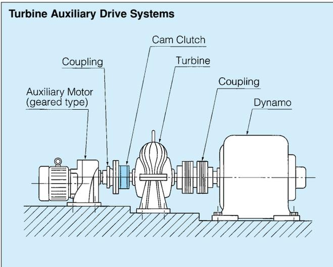
This example shows a Cam Clutch installed in the auxiliary drive system of a steam turbine. The auxiliary drive system powers the turbine at low speed through the engaged Cam Clutch, until steam pressure accelerates the turbine to the Cam Clutch release speed. Then the cam automatically disengages and runs as a high speed ball bearing, because there is no mechanical contact in the clutch.
