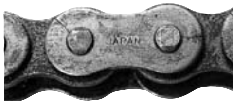
Hydrogen embrittlement cracking
