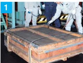
1 Chain is packaged in a special wooden box and delivered horizontally.
