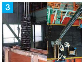
3 Chain is packaged folded on top of itself. Attach one end to a crane and lift out for easy removal.
