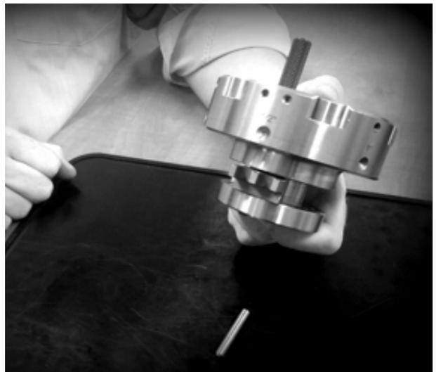
3) Take out the chain guide and replace it by a new chain guide.
