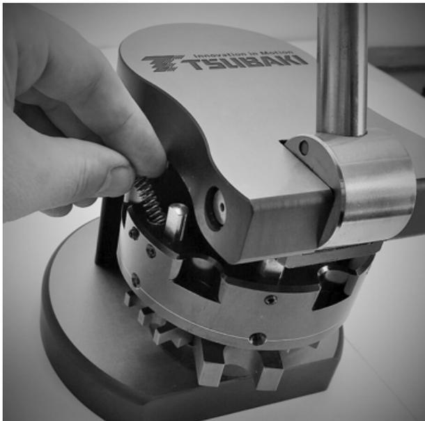
4) Turn the screw gently so that the cutting pin can be freely pressed down by a finger. Check if the cutting pin can move freely up and down. Adjust the screw until you reach a free movement of the cutting pin and at the same time ensure that it cannot be pulled up.
