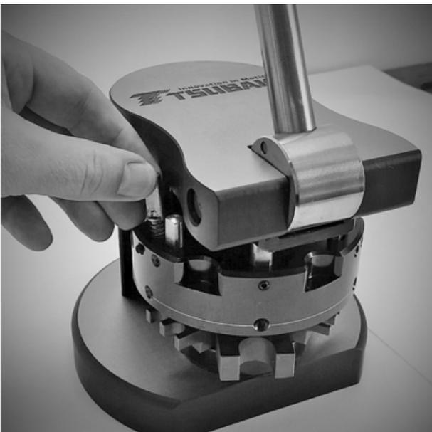
3) Pull the cutting pin up and return the spring to the hole.
