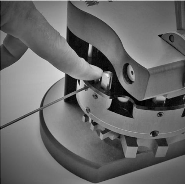
2) Then pull the cutting pin up from spring.
