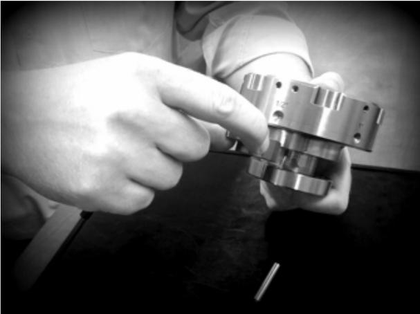
4) Press fit the fixing pins back (you can re-use the fixing pins).
