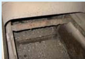
Fly Ash Conveyor: Dust Conveyor Under Boiler
